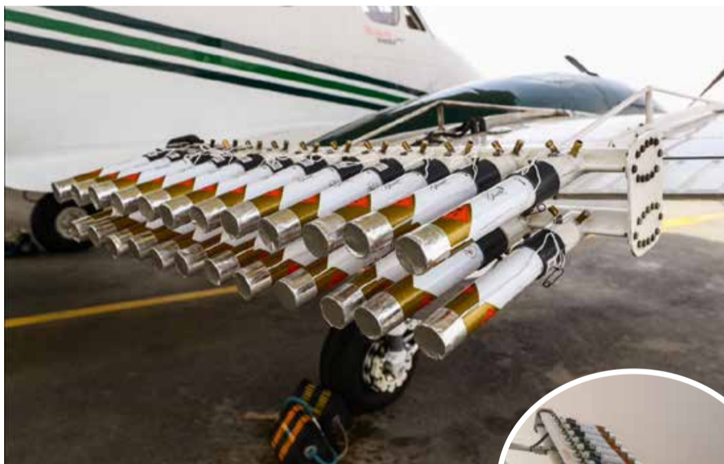
Hygroscopic flares are attached to an aircraft ahead a cloud seeding flight operated by the National Center of Meteorology, at Al Ain International Airport in Al Ain, in United Arab Emirates
