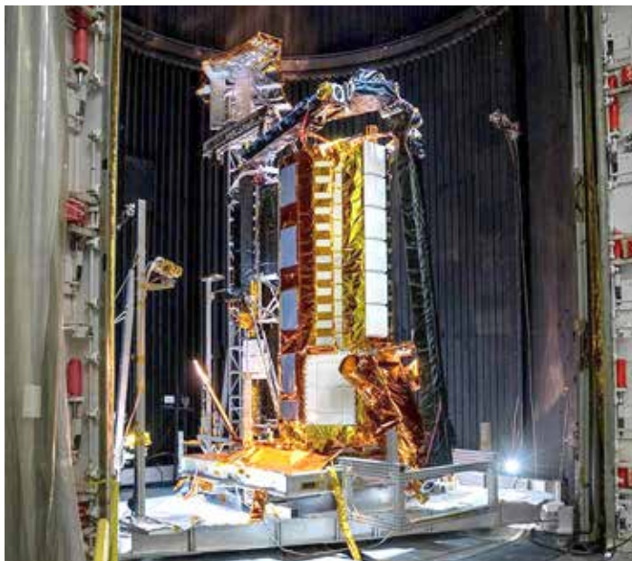
A part of the NASA-ISRO Synthetic Aperture Radar (NISAR) satellite resting in a thermal vacuum chamber, meant to mimic the conditions found in space, at NASA's Jet Propulsion Laboratory in August 2020
