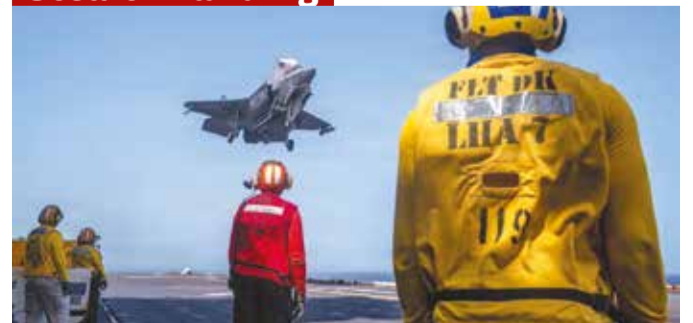
U.S. Sailors observe as a Marine Corps F-35B stealth fighter lands on the flight deck of USS Tripoli (LHA 7) while transiting the Arabian Sea. The F-35B is designed to perform short takeoffs and vertical landings.
