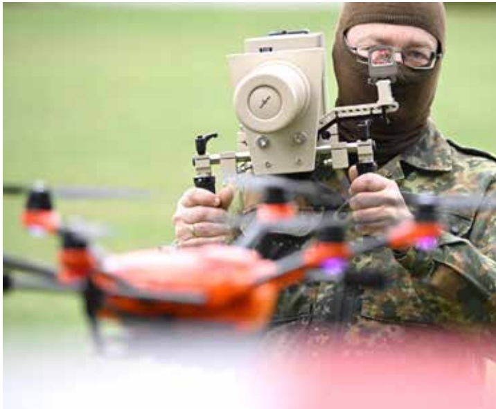
A soldier of the German armed forces Bundeswehr demonstrates the use of a handheld HP 47 drone jammer
