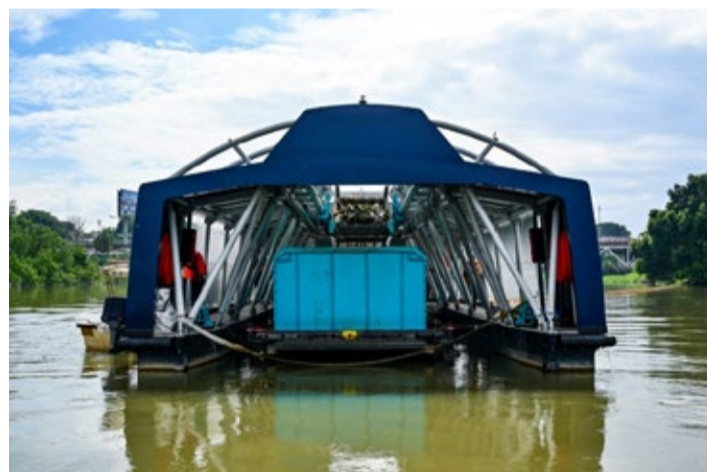
The Interceptor barge can collect up to 50 tons of waste a day
