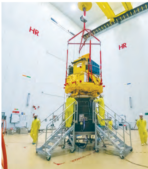
The Smile spacecraft (gold) fixed to a Vega-C rocket adaptor (black cone) in Kourou, French Guiana, in preparation for liftoff from Europe's Spaceport.
