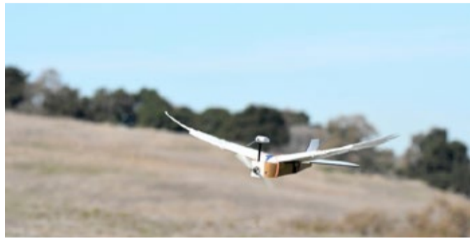
A radio-controlled robot with wings made with 40 real feathers
