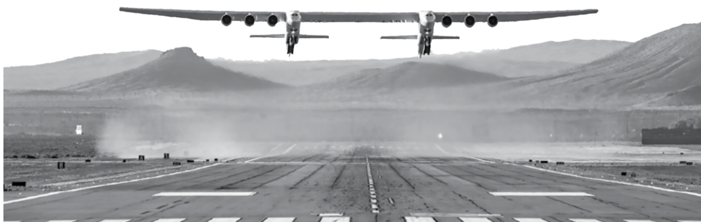
The world's largest airplane -- a Stratolaunch behemoth with two fuselages and six Boeing 747 engines -- made its first test flight in California.
