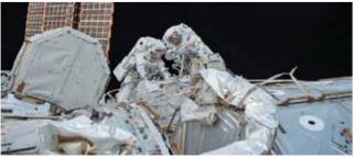
NASA astronauts outside the International Space Station to grease the robot arm's new hand.
