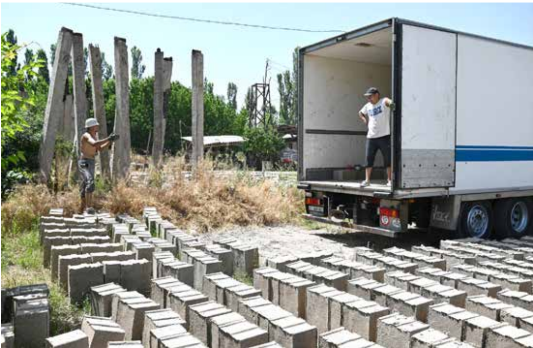
A view of the production facility of rice construction blocks, made mostly of rice husks - a byproduct of rice processing, in the Batken region in southern Kyrgyzstan
