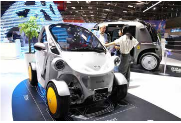
A PIX Beastie mini electric vehicle with a 3D printed unibody chassis
