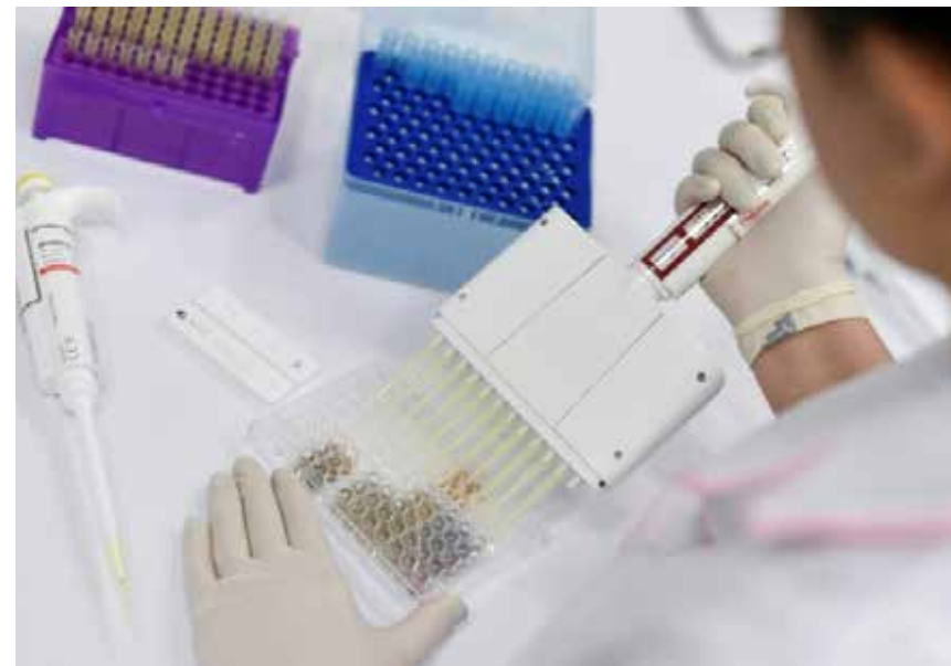
A lab technician inserts reagents into a plate with a patient's samples to perform COVID-19 PCR tests
