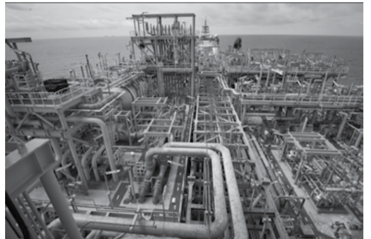
A view of the Kaombo Norte, an oil tanker converted into a FPSO vessel
