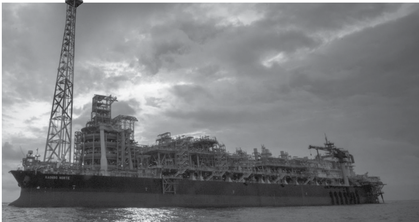
A view of the Kaombo Norte, a Floating Production Storage and Offloading vessel (FPSO), a project operated by Total, the French multinational oil company
