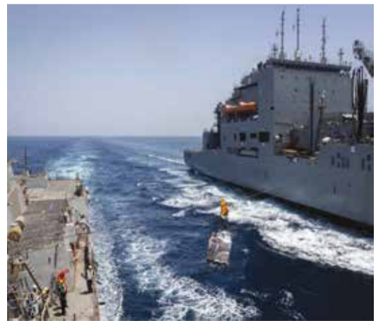
USNS Wally Schirra (T-AKE 8) replenishes the guided-missile destroyer USS Delbert D. Black (DDG 119) while at sea. Underway replenishments allow U.S. Navy ships to receive fuel, food, munitions, and essential supplies.
