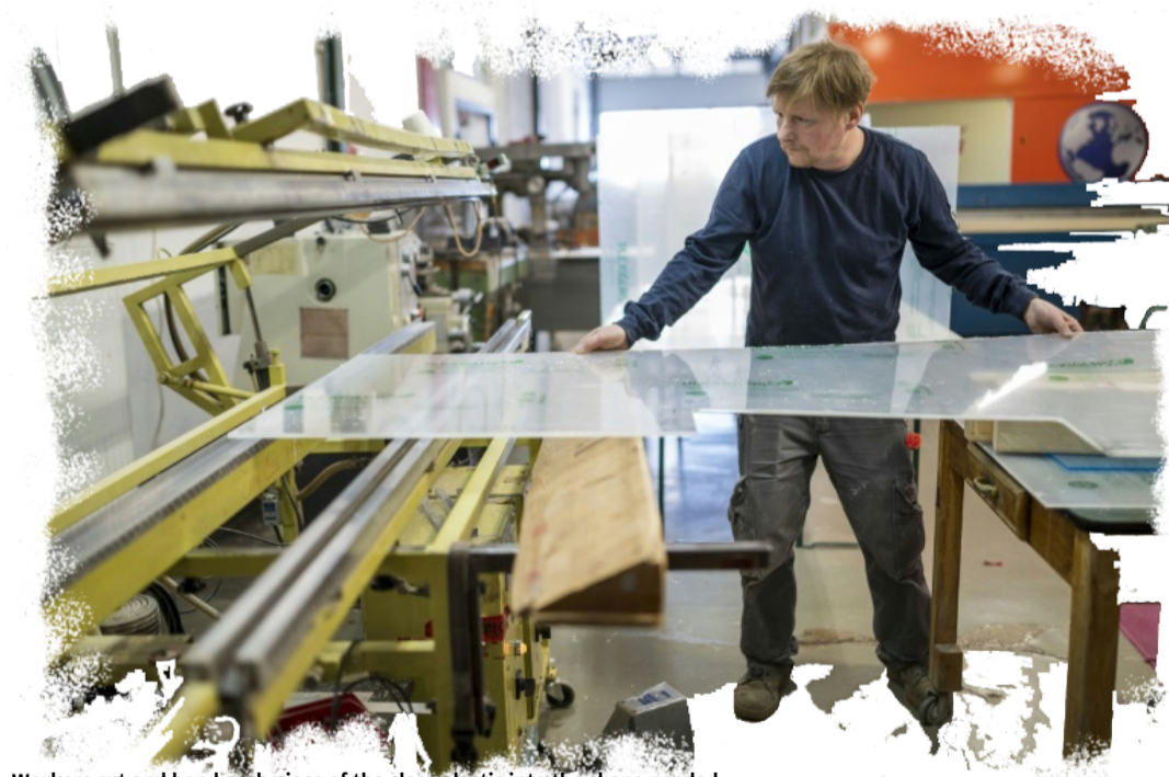
Workers cut and bend each piece of the clear plastic into the shape needed
