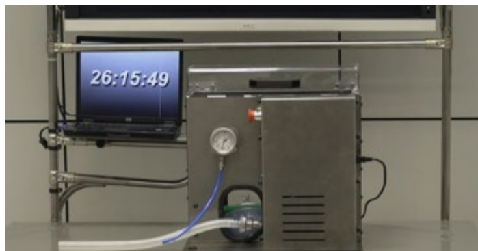
A mechanical ventilator being developed by Spanish automobile manufacturer SEAT at the company's Martorell factory using a windscreen wiper motor
